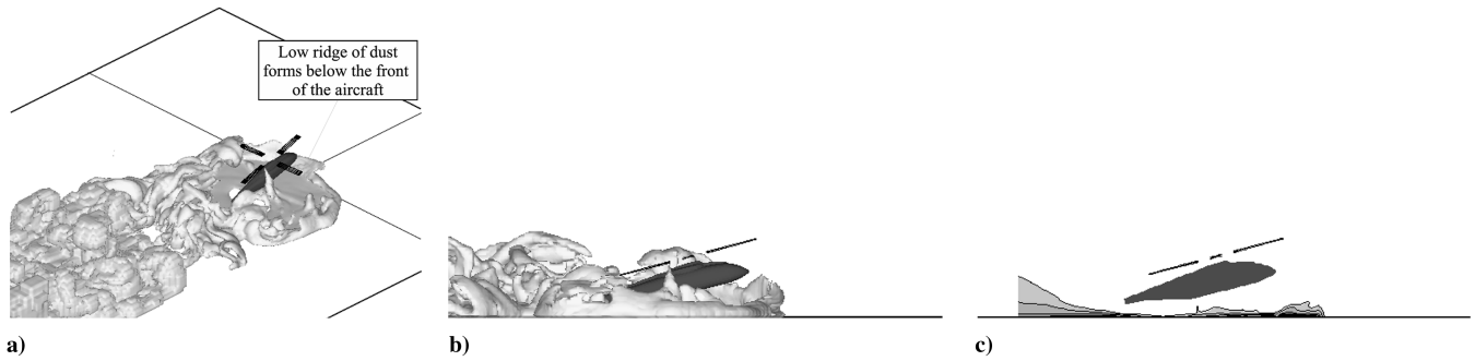
Fig. 12 VTM-predicted dust distribution surrounding a helicopter with single main rotor configuration ( \mu^* = 0.47 ).
